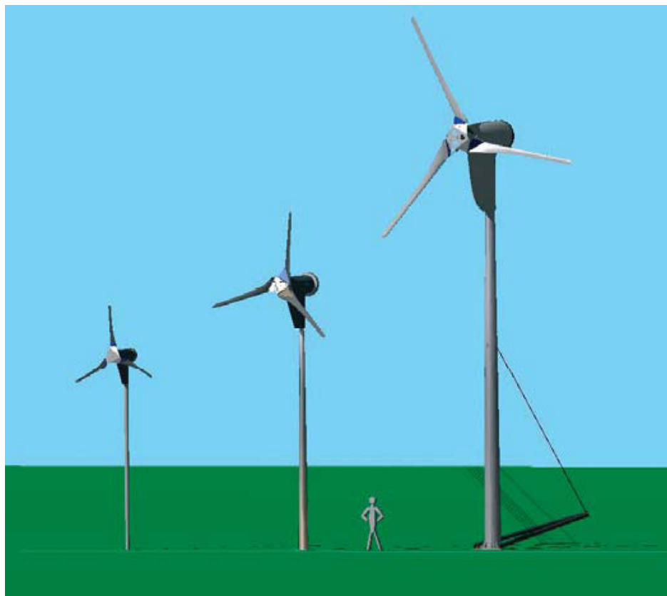
From right to left Proven 2.5kW on a 6.5m tower. Proven 6kW on 9m tower, 6ft tall man and a 15kW on 15m tower
