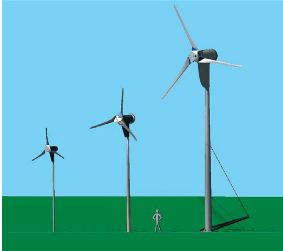
From right to left Proven 2.5kW on a 6.5m tower. Proven 6kW on 9m tower, 6ft tall man and a 15kW on 15m tower
